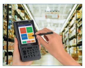
The built-in wireless LAN module (R- and CR-models only) enables safe high-speed and real-time communication in either the 802.11b or 802.11g standard with data transfer rates of up to 54 mbps. So an upcoming upgrade of existing WLAN networks will be no problem with using the IT-600.
