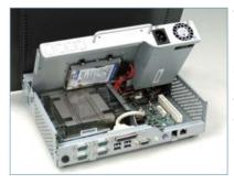
The C67 MB with Sandy Bridge CPU processors i7/ i5 series to provide AMT (Active Management Technology) and virtualization capabilities
